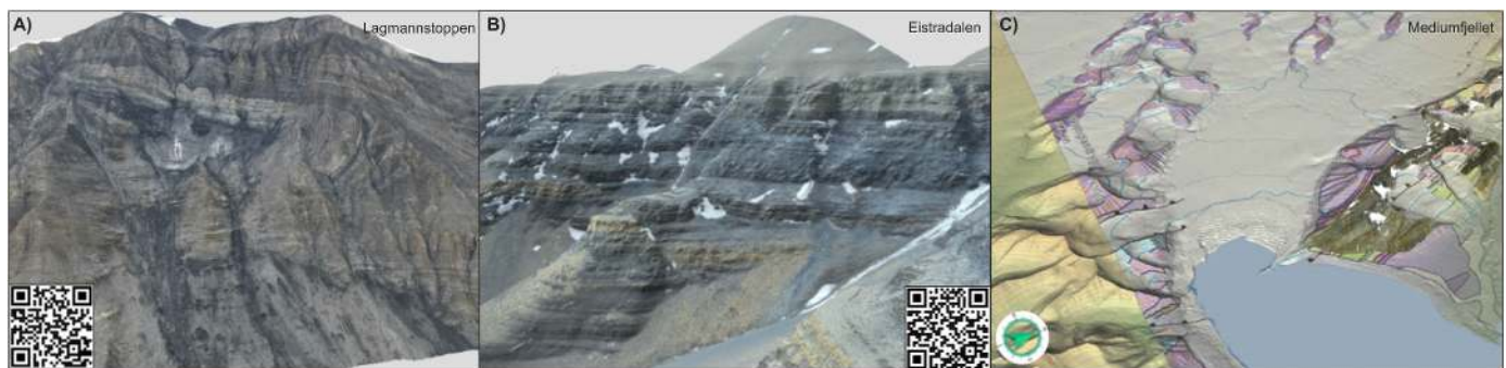
Fig. 8. Examples of two digital outcrop models from Svalbox and one from V3Geo. At Lagmannstoppen ( Lord et al., 2021 ) in western Spitsbergen the Alkhornet Formation is heavily deformed and is a good example of thick-skinned tectonism in the WSFTB. At Eistradalen ( Betlem and Rodés, 2021 ) in eastern Spitsbergen only the sedimentary cover is affected by faulting. The QR codes point to downloadable and interactive versions of the DOMs (also listed in Table 1 , along with a number of other relevant DOMs). The Mediumfjellet model from V3Geo is placed in context by incorporating a DEM draped by a geological map and was analysed as part of the AG222 course at UNIS ( Senger et al., 2021c ).
